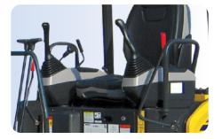
**Neutral Engine Start System** Locks out drives and hydraulics during machine start up.
